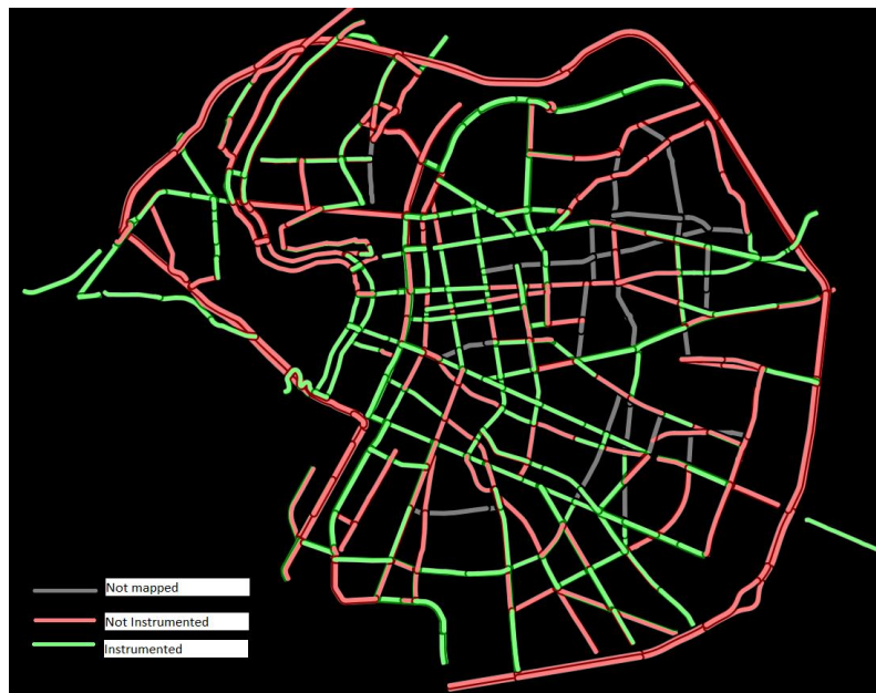
Figure 11. Lyon CRITER segments; green segments are those for which sensor data is available (instrumented), red segments are un-instrumented, grey segments to minor un-mapped streets.
